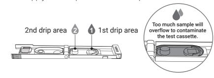
**Step 6** Close the test cassette, and lock it.(push the locker to the end)
