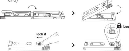
**Step 6** Insert the cassette into the slot and push it to the end.
